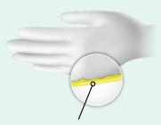
A coating is applied over the glove former to seal any micro-defects, creating a smooth finish and delivering a consistent thickness across the glove. This minimizes irregularities that may later result in pinholes
